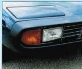
Unlike the 365 GTB/4 Daytona, all 365 GTC/4s came with pop-up headlights regardless of where they were sold.
