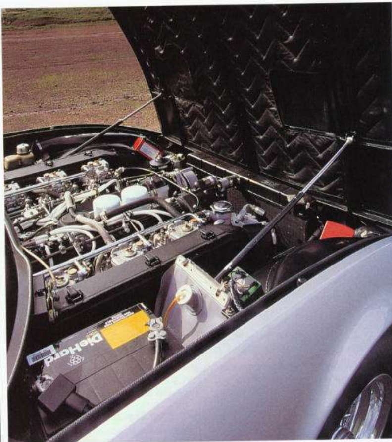
EXPENSIVE VIEW: The C/4's engine is costly to service and repair. "Those side draft Webers are a pain in the neck," says FORZA's tech consultant, Tony Palladino.
