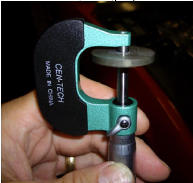
After measurement, carefully replace the shim back in its bucket, making sure to keep the “business” end facing upward toward the cam (don’t get your fingers under the cam, in case the wedge gives way!). It will take a little jiggling to get it to seat properly, and you may have to tap it with a soft brass punch on alternate sides to get it to seat. It is properly in place when you can again rotate the shim in its bucket with your finger.
