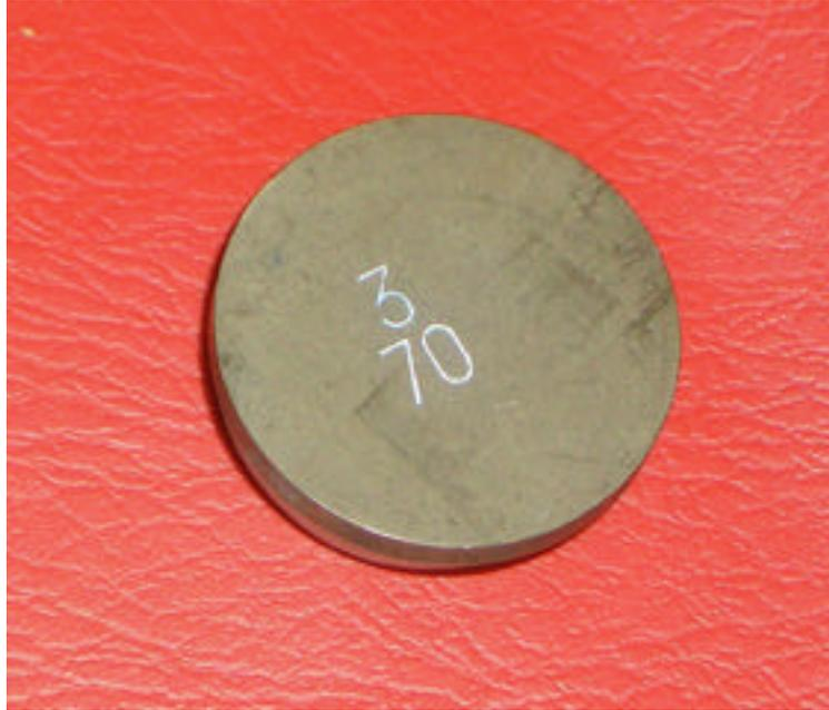
Don't take this as gospel, however, and go ahead and measure with your micrometer. Most likely your micrometer will be in inches. While you have the shim in your hand, go ahead and make the conversion from your measurement in inches, to millimeters, and compare with the value stamped on the shim, as a double-check. (multiple inch measurement by 25.4 to get equivalent millimeter).
